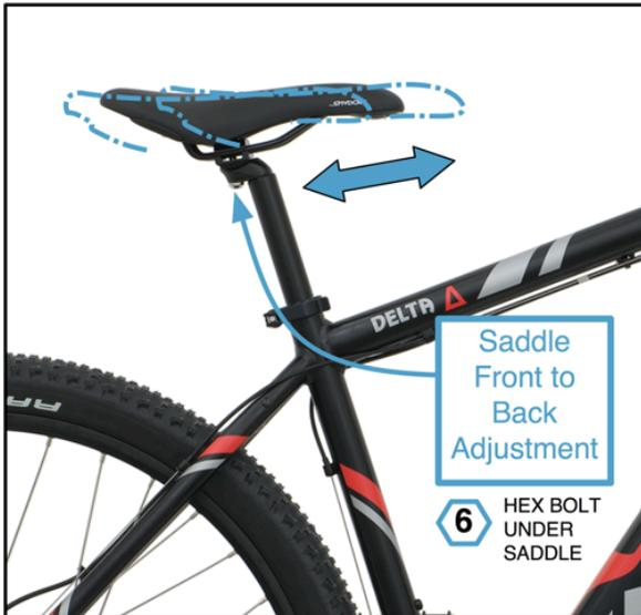
The saddle can also be adjusted frontwards or backwards on its mount. Take care with all fasteners after adjustment to ensure that they are safely tightened to avoid movement and potential injury whilst riding.
